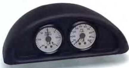
Exclusive Saleen twin gauge pod (deletes clock), featuring boost and fuel pressure gauges.
