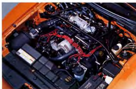
4.6 liter, 281 cid modular engine. Features single or dual overhead cam and distributor-less ignition system with a 5-speed manual or 4-speed automatic transmission.
