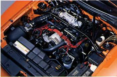
New for '96! 4.6 liter, 281 cid modular engine. Features single overhead cam and distributor-less ignition system. 220 HP with a 5-speed manual or 4-speed automatic transmission.
