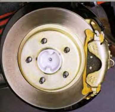
Four-wheel disc brakes with 5-lug bolt pattern
